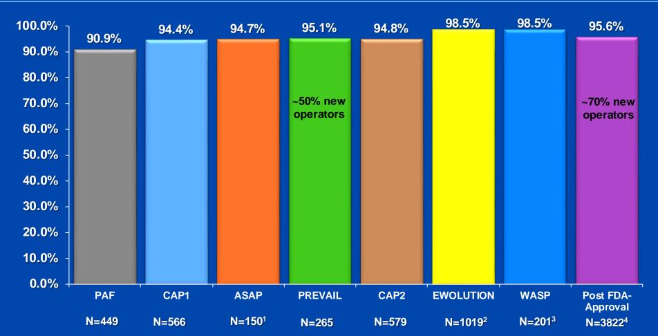
Implant success defined as deployment and release of the device into the LAA; no leak ≥ 5 mm
